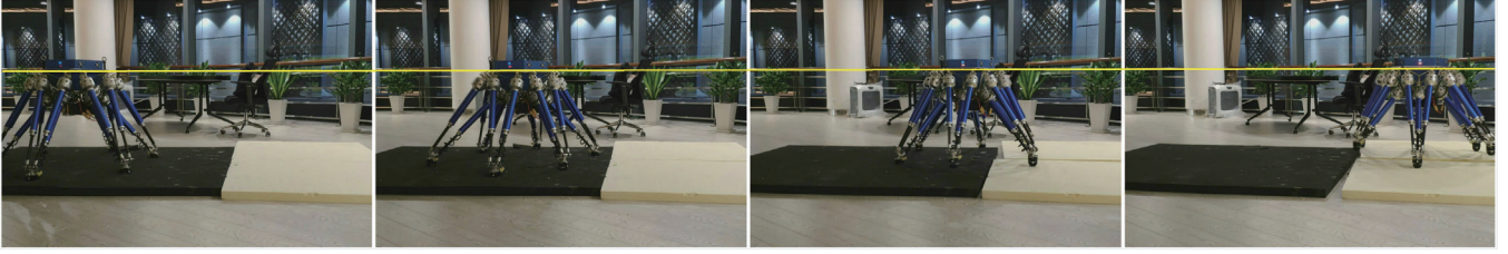
Fig. 6. The robot traverses from the black, soft sponge to the yellow, hard foam by a 3-3 gait. DPPF with the prior from ground material segmentation is utilized for real-time stiffness estimation. With the estimated stiffness, the contact force can be maintained more accurately and the robot's body relative to the ground can be kept with a constant height and posture.
